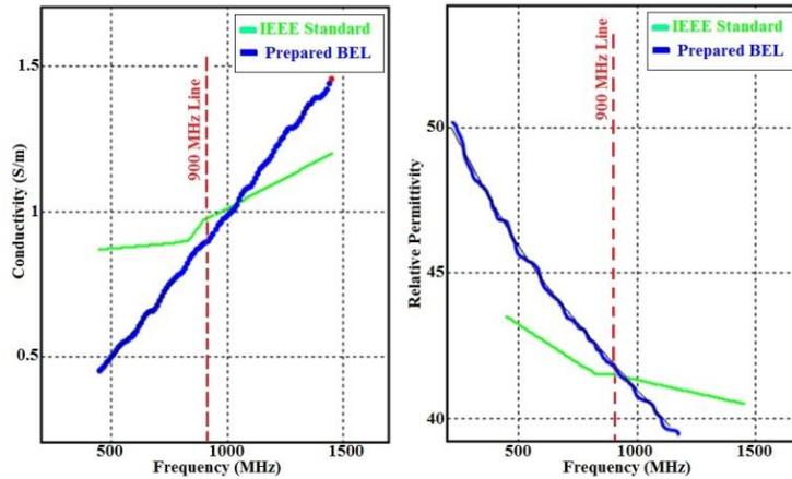
Fig. 1. 900 MHz HEL Performance versus IEEE 1528 Standard
