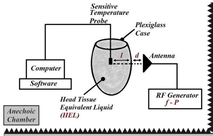
Fig. 2. Measurement Setup.
