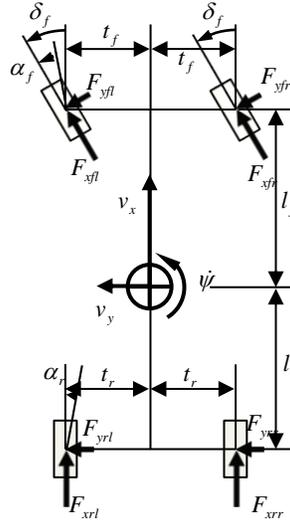
Fig. 1. Plane two track model
