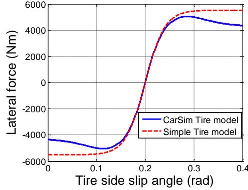
Fig. 2. Comparison of a simple tire model with the Carsim tire model
