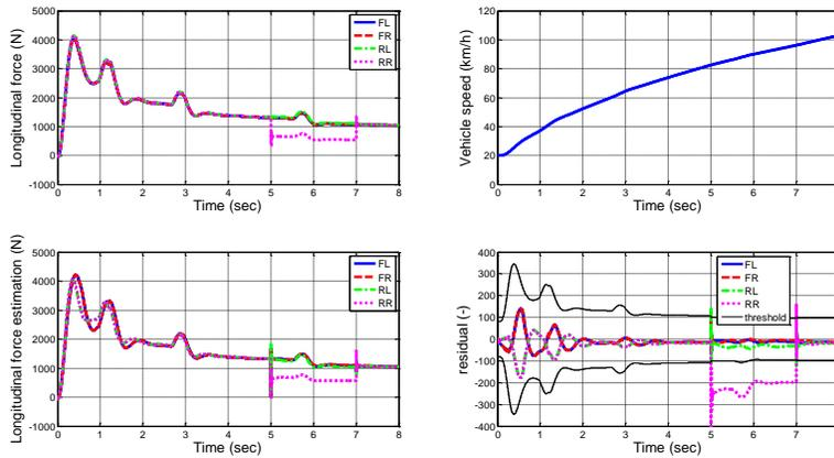
Fig. 5. Simulation result (Initial speed 20km/h, throttle=0.5 acceleration)
