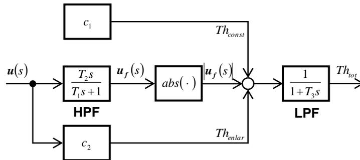
Fig. 3. Structure of the adaptive threshold generator
